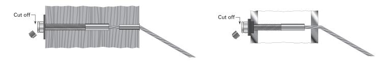
**2.** Twist the cap over the locknut.
