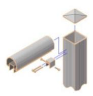
D. Measure from inside of post to inside of post and cut RFX100 top rail & BR100 bottom rail (bottom rail optional) to fit. Set top and bottom rails on previously installed RCBs and attach with screws from both sides.
