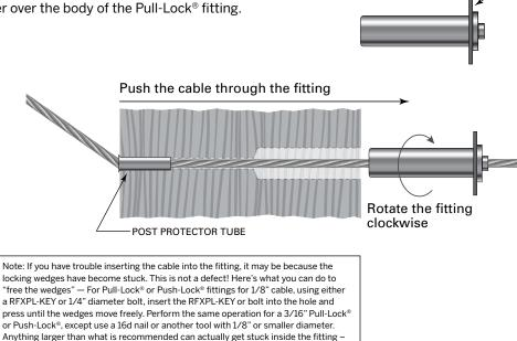
**3.** Push the Pull-Lock<sup>®</sup> fitting along the cable and firmly into the hole in your post. Pull on the cable (cable gripping pliers are helpful for this) to create as much tension as possible as you seat the Pull-Lock fitting into the hole.
