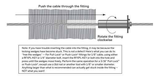
**3.** Push the Pull-Lock<sup>®</sup> fitting along the cable and firmly into the hole in your post. While holding the Pull-Lock<sup>®</sup> fitting against the end post, pull the bare end of the cable to remove as much slack in the cable as possible.
