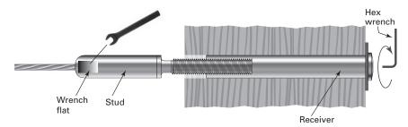
**2.** Finish tensioning the cable at the post with tensioning terminal by holding the cable securely to prevent it from turning while you turn the Receiver with a hex wrench. Be careful to protect the cable from damage while tensioning.
